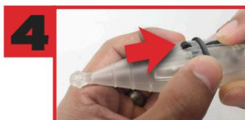
**4** Keep rolling ring over trigger and on to lever. Lock lever by pushing trigger toward large opening while continuing to hold lever down.
